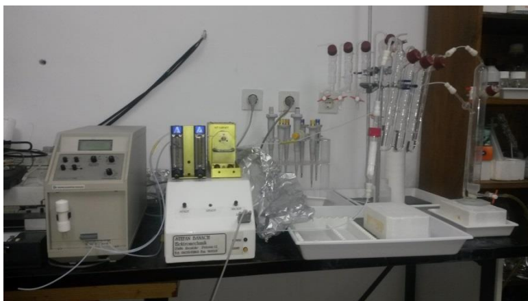
Slika 1.5.1.1. Atomska apsorpcijska spektrometrija hladnih para (CV-AAS – engl. cold vapour atomic absorption spectrometry; Mercury Monitor 3200, Thermo Separation Products, SAD)
