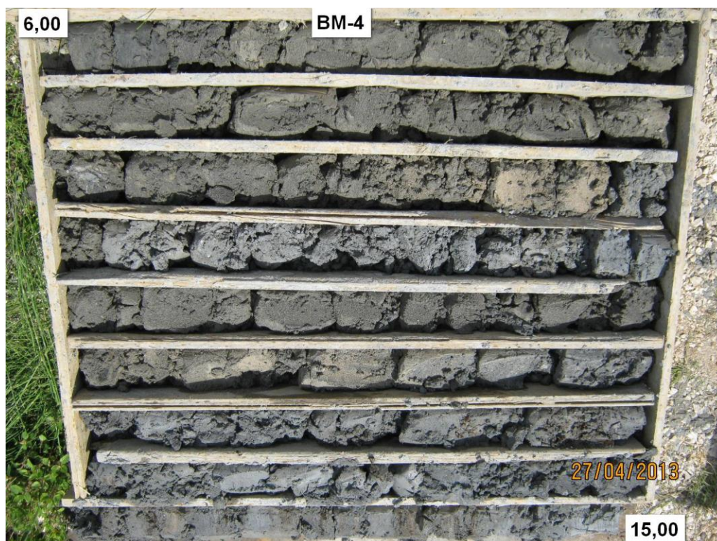
Slika 2. Jezgra istražne bušotine BM-4 (6,0-15,0 m)
