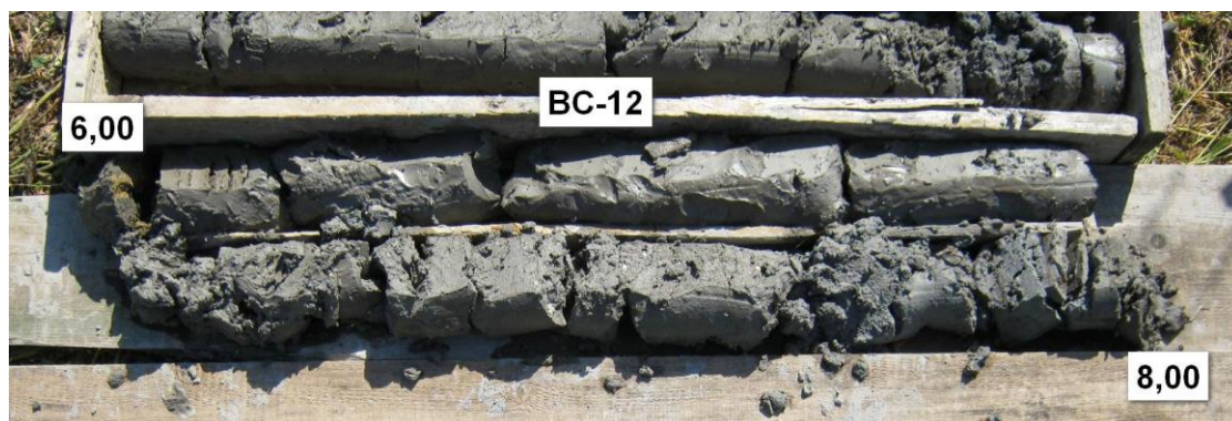
Slika 2. Jezgra istražne bušotine BC-12 (6,0-8,0 m)
